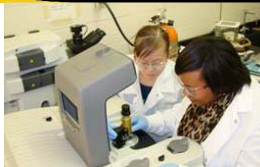
Chemistry students using Fourier Transform Infrared Spectrometer to analyze structure of a chemical compound
